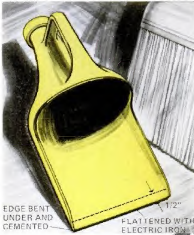
DUSTPAN from an empty Clorox jug is still another way to utilize those handy plastic containers. After cutting to shape, flatten the bottom with an electric iron set for "nylon."— M. A. Elliot, Hilo, Hawaii
